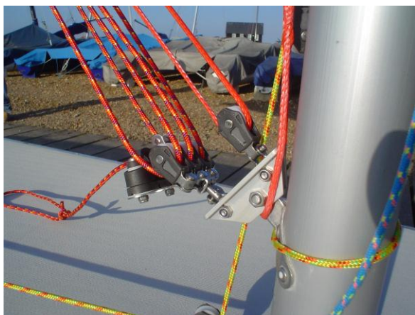
Mast base kicker tang with base plate fitted
