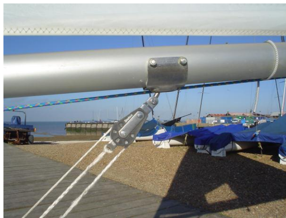
Top block located into boom fitting
